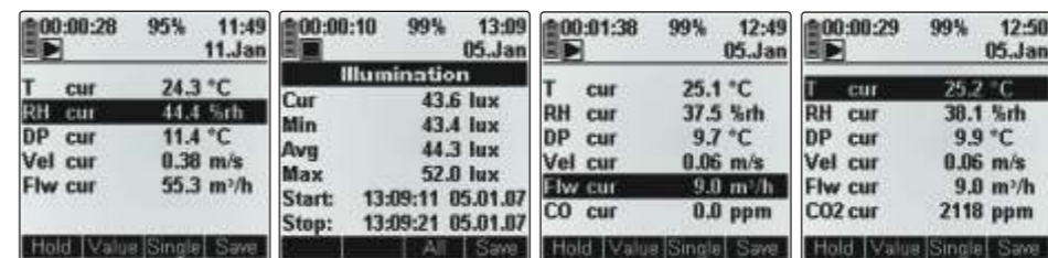
Measurement with universal microclimatic, illuminance, CO and CO 2 probes.
